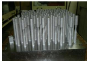
Fig. As-built and vertical cylindrical bars
